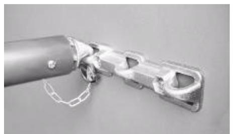
**Fig.4 Breast bar pin end fitted to trailer side panel**
